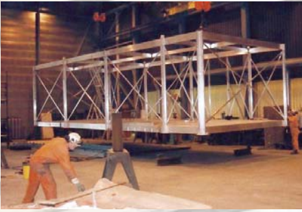
STRUCTURAL FRAMEWORK OF STATFJORD A MODULES (ALUMINIUM)
